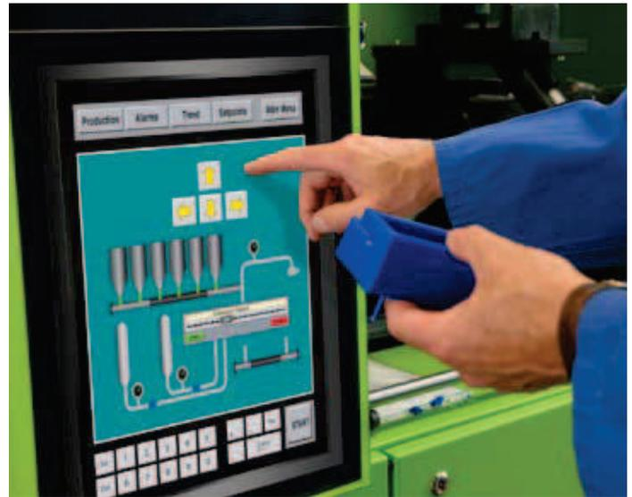
The C1500SS display has several bezel options that provided the OEM's customers with the ability to customize ingress protection based on their needs. For those with a NEMA 1 rating (for dust contamination), the 3M MicroTouch Slimline and Contour bezels (see Figures 1 and 2) were the best solution. For customers needing a liquid ingress protection rating of NEMA 4, the 3M MicroTouch Industrial Flange bezel (see Figure 3) provided the necessary sealing level.
