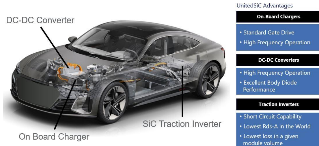
Figure 1: The main applications of SiC FETs and Diodes in EV applications. The main advantages of using UnitedSiC FETs in these applications are summarized on the right.
