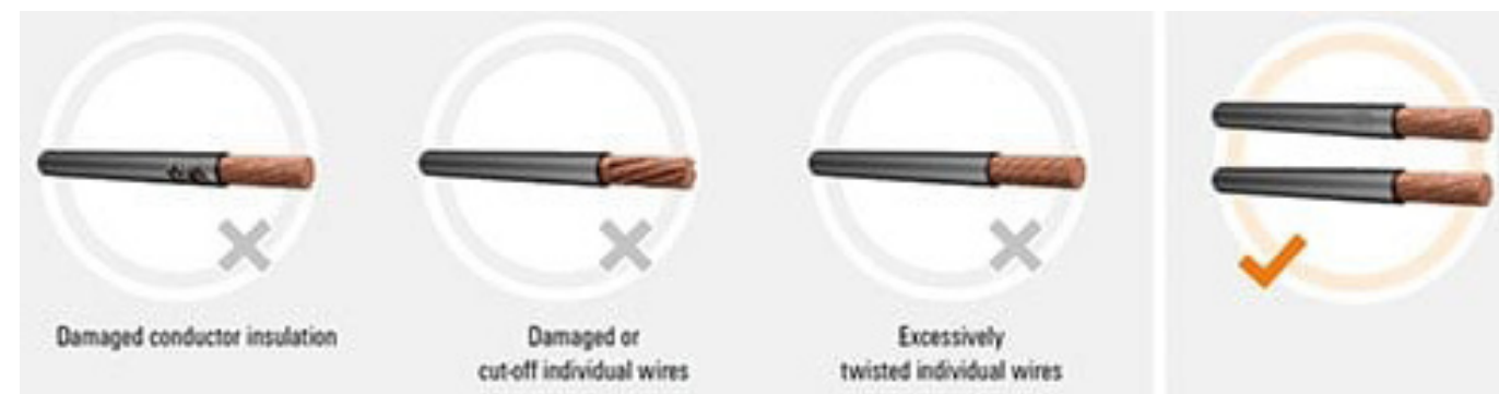
Figure 7: Shown are three examples of insulation stripping errors as well as a properly stripped wire. Image source: Weidmüller Interface GmbH & Co.
