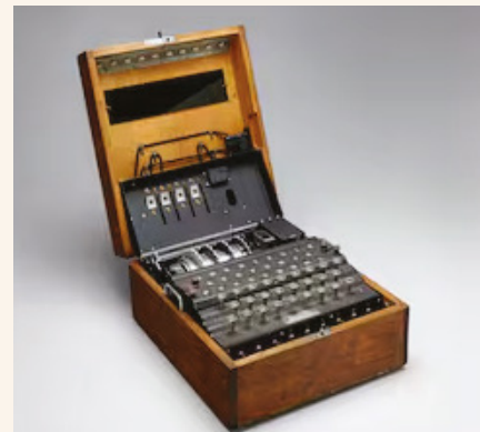
Early Enigma cipher machine used by German military forces, an electromechanical device that encrypted communications using rotating cipher rotors.
