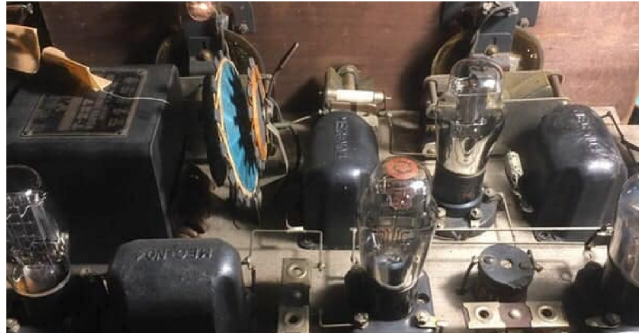
Example of the insides of a 1920s radio set.
