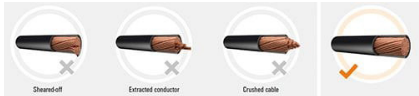
Figure 6: Shown are the three ways a wire can be improperly cut, as well as the appearance of one done correctly. Image source: Weidmüller Interface GmbH & Co.
