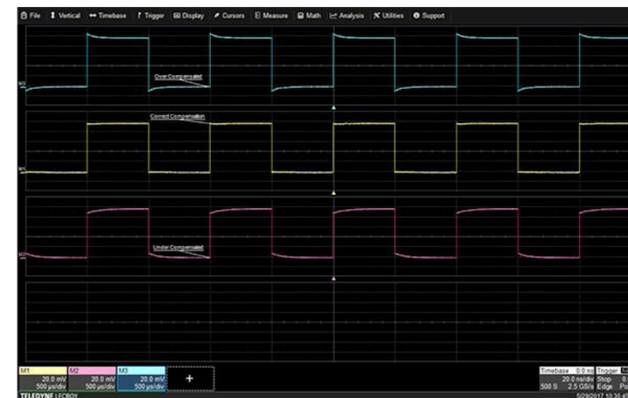
Figure 3: Low frequency compensate the probe by adjusting the compensation adjustment to obtain a square corner on the CAL square wave, as shown in the center trace. Image source: DigiKey
