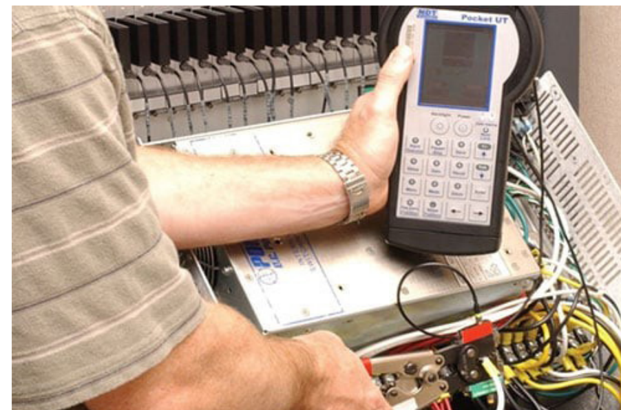
Figure 8: This portable instrument developed by NASA can non-destructively identify crimp quality and problems both good crimps and the many types of bad crimps in real-time. Image source: NASA
