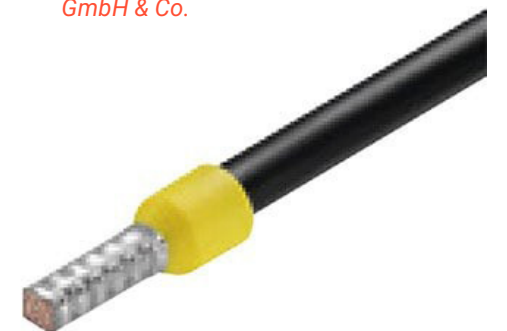
Figure 3: This crimped wire-end ferrule is available in many sizes and has a plastic collar as an additional insertion aid due to the conical shape in the inner diameter of the collar.
